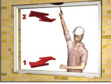
Place a Winbag at the top and adjust in and out by pushing and pulling the window until it is at level with the facade.
