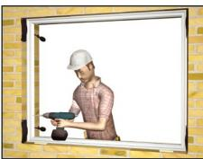
Fasten the window, while it is kept in place by the Winbags. Remove the Winbags by deflating them. The joint is now completely empty and ready for sealing.
